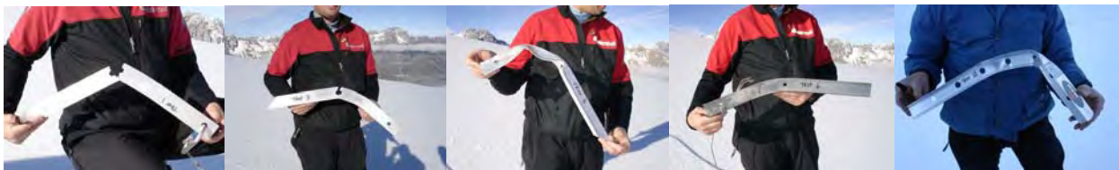
Five upright topclips in knife hardness -10^{\circ} C snow. Left to right:- Test 1 Al alloy (6261 T6) failed in shear at 9.4 kN. Test 3 Al Alloy failed in compression at 6.7 kN, Test 5 was open part of V to load and failed at 4.4 kN through buckling of the stake. Test 6 was 3mm mild steel which failed in shear at 11.3 kN. Test 12 was a MSR coyote that failed in compression 7.8 kN
